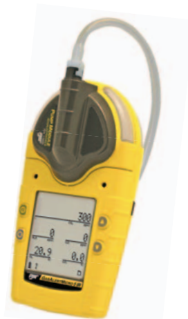
GasAlertMicro 5 IR with integrally attached pump
