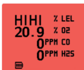
Red display in alarm conditions
